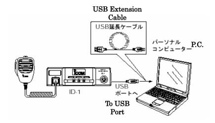
The ID-1 is connected to the PC by the USB cable.
